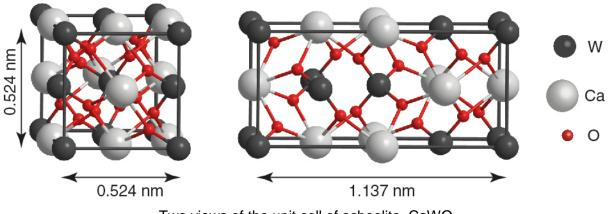
Two views of the unit cell of scheelite, CaWO<sub>4</sub>.
